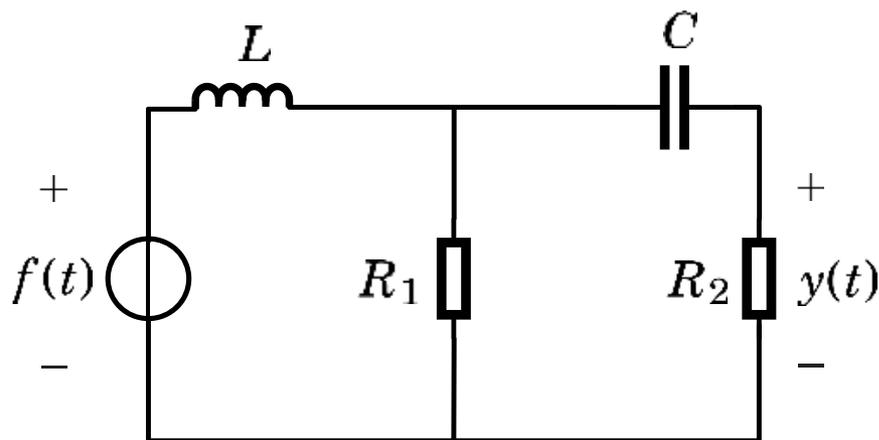
$$L \left( \frac{1}{R_1} + \frac{1}{R_2} \right) y''(t) + \left( \frac{L}{R_1 R_2 C} + 1 \right) y'(t) + \frac{1}{R_2 C} y(t) = f'(t)$$
