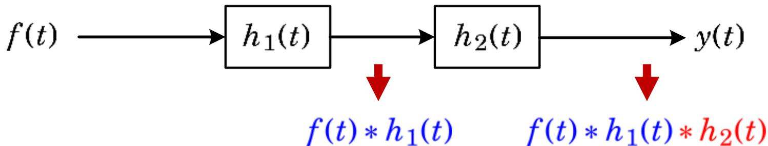
$$y(t) = f(t) * [h_1(t) * h_2(t)] \quad \text{结合律}$$
