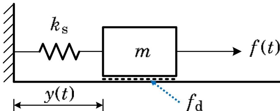
$$f_i(t) = m \frac{d^2 y(t)}{dt^2} \quad f_f(t) = f_d \frac{dy(t)}{dt} \quad f_k(t) = k_s y(t)$$
