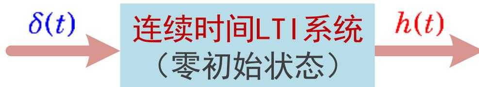
$$\left\{ \begin{aligned} & h^{(n)}(t) + a_{n-1}h^{(n-1)}(t) + \cdots + a_1h'(t) + a_0h(t) \\ & = b_m\delta^{(m)}(t) + b_{m-1}\delta^{(m-1)}(t) + \cdots + b_1\delta'(t) + b_0\delta(t) \\ & h^{(i)}(0^-) = 0, \quad i = 0, 1, n-1 \end{aligned} \right.$$
