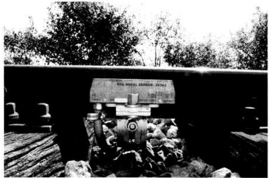
Fig. 10. 2 Modern type axle counter detection point
